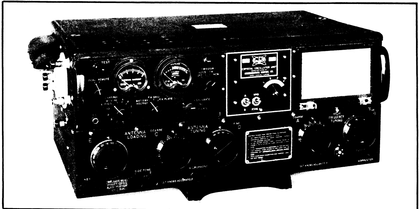
Figure 1-2A—Radio Transmitter T-47A/ART-13 with Oscillator CDA-T Installed
